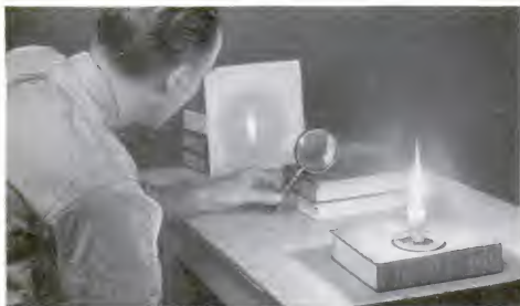
How an ordinary lens refracts light of various colors unequally
